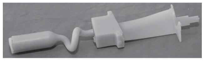
Fig. 5. Model kit from casting wax
